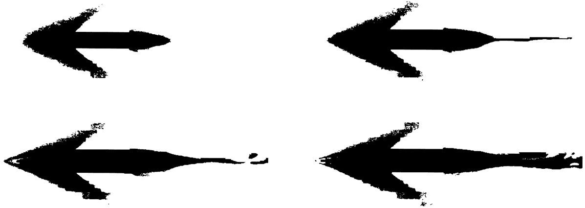
Figure 6. Longitudinal slices of density field for Mach 2.33 flow past a cone-cylinder, with a semi-apex angle of 8.58 degrees.
