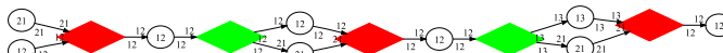
Fig. 8. An extended merge event: Two cells (initially labeled 12 and 21) merge and split twice before ultimately merging. These are inherent instabilities in segmenting by thresholding caused by saddles very close to the cut-off.
