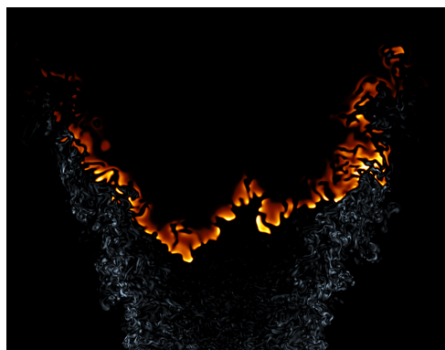
Figure 4: Composite image (cropped in near the flame/nozzle region) simultaneously shows the OH intensity (in orange) and the magnitude of vorticity (in grey). Turbulence approaches the flame from the core of the inlet nozzle at the lower domain boundary, and is generated by shear in the swirling flow region.
